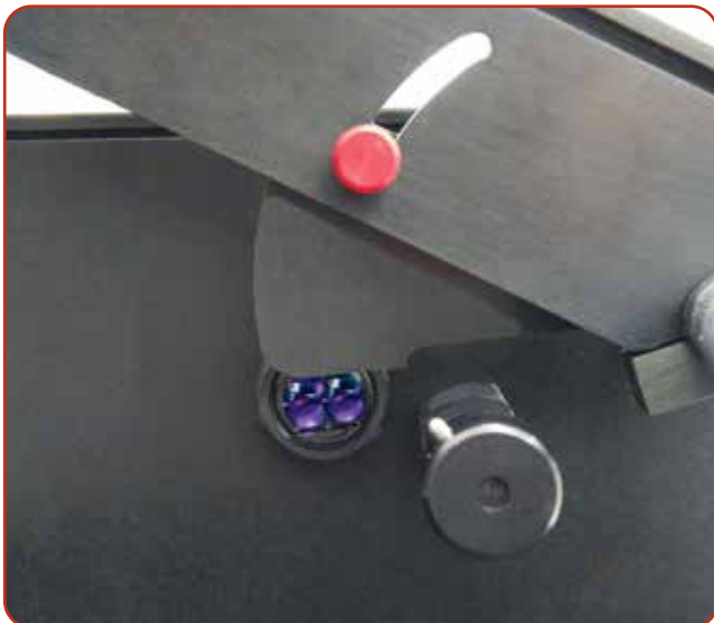
Optical shut-off sensor with adjustable stop
